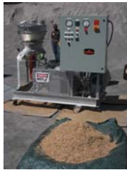
A machine chips the woody debris (biomass) to specific dimensions for the maximum yield of oil and char.
